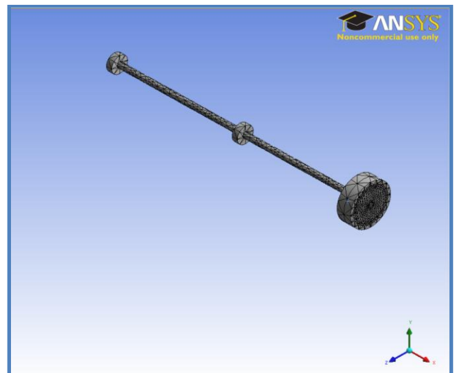
Fig. 2 Finite element model (gyroscopic geometry) ANSYS work bench (three dimensions).
